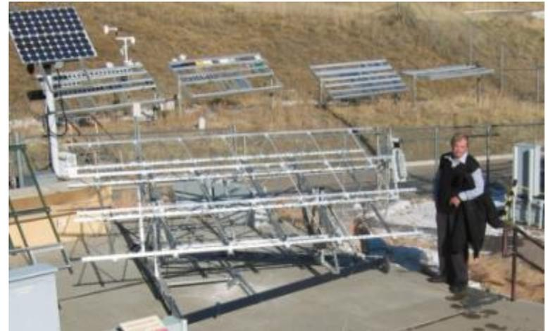
A version of sun tracker for 1 kWp installed in NREL (Golden, Colorado; Dec. 2004)
