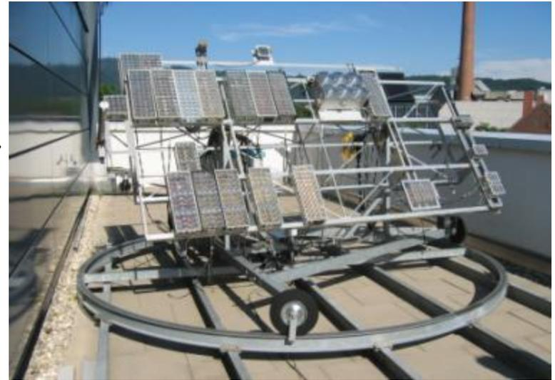
The same tracker after four years of operation on the roof of the Fraunhofer-ISE
