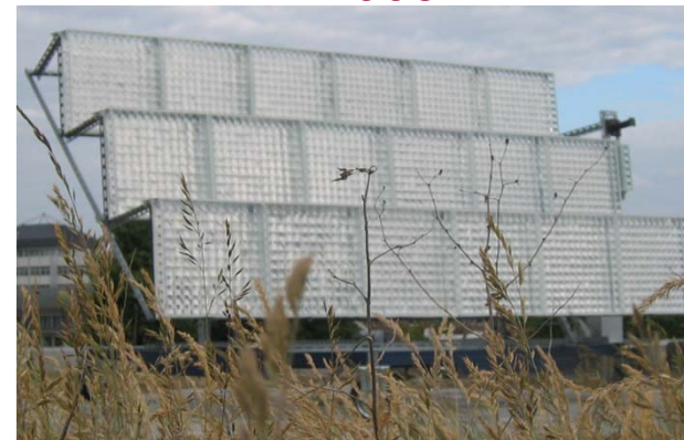
Fresnel lens panels (“silicone on glass” design)
