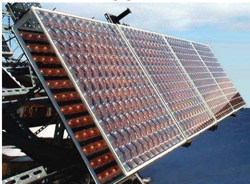
Fresnel lens panels (“silicone on glass” design)
