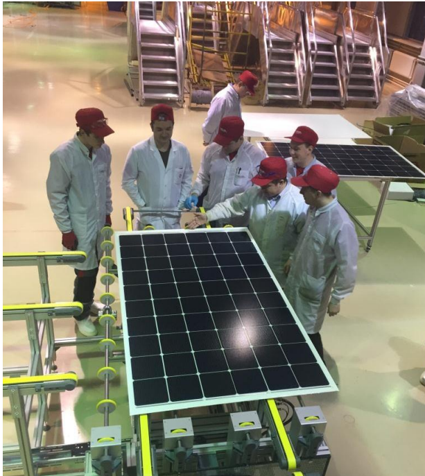
First modules assembled with using of SmartWire technology (from Meyer Burger) show power above 290 W
