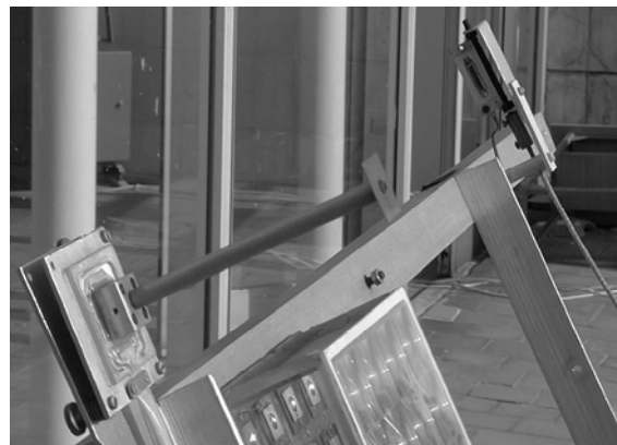
Figure 5: Main sun sensor (on the left) and additional one (on the right) mounted on the 0.2 kW tracker.
