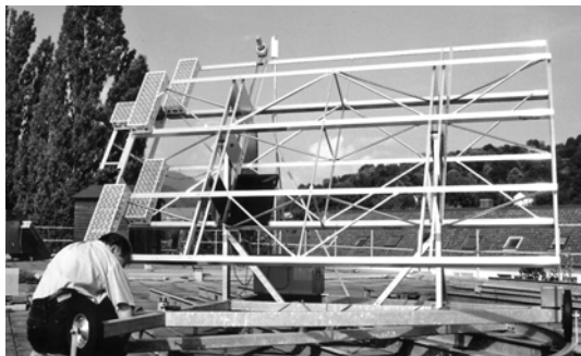
Figure 6: The 1 kW tracker with four full size-concentrator modules. One reduced-size module serves as a power supply for the tracking (Fraunhofer ISE, Germany).
