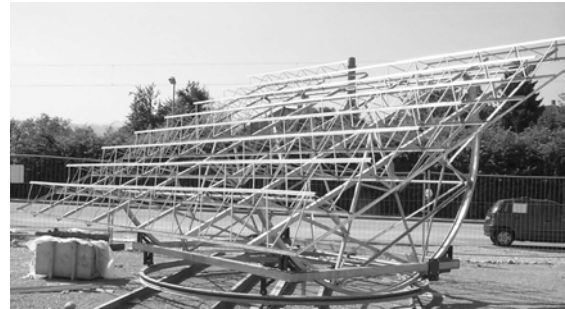
Figure 7: The structure of the 5 kW tracker (Freiburg).
