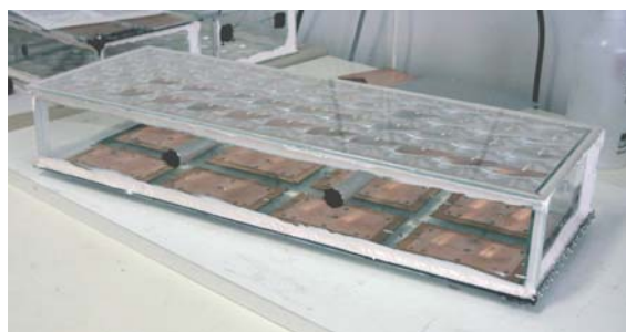
Figure 1: Photograph of a FLATCON TM module. 48 Fresnel lenses concentrate the sunlight to dual-junction cells with a diameter of 2 mm. A geometrical concentration ratio of 500 is realised. The aperture area of one FLATCON TM module is 768 cm 2 .
