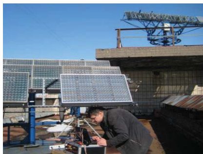
FIGURE 6. One of the full-size modules (288 pcs of 40x40 mm 2 lenses and cells) at outdoor I-V measurements.
