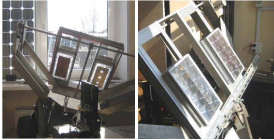
FIGURE 3. Back and front pictures of two test modules (8 lenses of 60 \times 60 \text{ mm}^2 in size) with parallel-connected triple-junction InGaP/GaAs/Ge solar cells mounted on copper and steel heat spreaders: sunlight illumination intensity of 610 \text{ W/m}^2 ; no wind; ambient temperature T_{\text{amb}} = 23 \div 24^\circ\text{C} .
