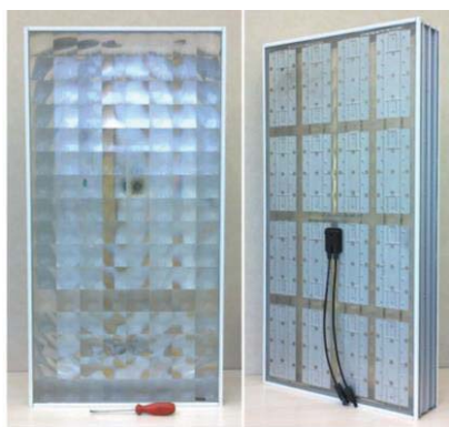
FIGURE 5. Pictures of the front and rear sides of a SMALFOC module with 128 lenses of 60x60 mm 2 and 16 integrated PV units.
