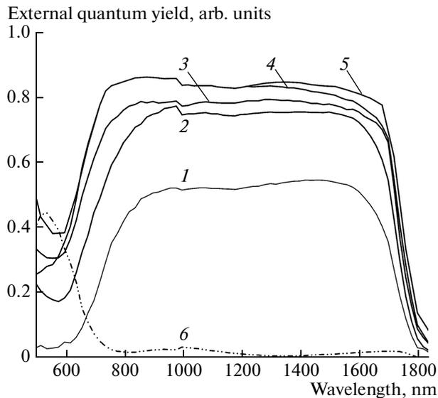
**Fig. 1.** Spectral characteristics of the external quantum yield of GaSb photovoltaic cells with various  $p-n$ -junction depths: (1) 1.1, (2) 0.9, (3) 0.62, (4) 0.32, and (5) 0.14  $\mu\text{m}$ ; (6) reflectance spectrum of an illuminated GaSb surface with a two-layer ZnS + MgF<sub>2</sub> antireflection coating.
