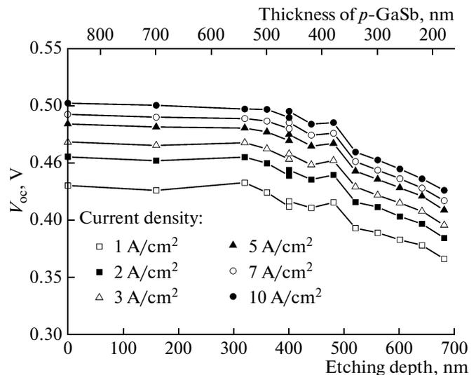
**Fig. 4.** Open-circuit voltage of a GaSb photovoltaic cell vs. the thickness of the diffusion emitter (upper scale) and the etching depth of the structure (lower scale) at various generated photocurrent densities.
