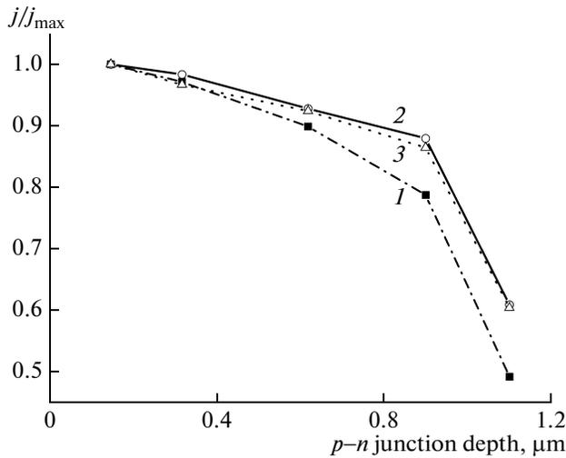
**Fig. 2.** Dependence of the normalized short-circuit photocurrent density  $j/j_{\max}$  for structures with various  $p-n$ -junction depths: (1)  $\Delta\lambda_1 = 500\text{--}1840$  nm, (2)  $\Delta\lambda_2 = 900\text{--}1840$  nm, and (3)  $\Delta\lambda_3 = 1180\text{--}1840$  nm.
