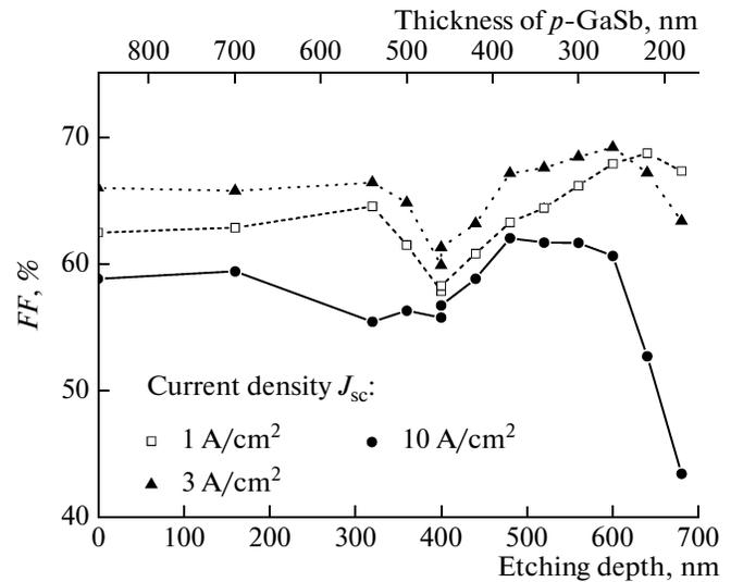
Fig. 6. Fill factor of the current–voltage characteristic vs. the etching depth and diffusion-emitter thickness at different generated photocurrent densities.
