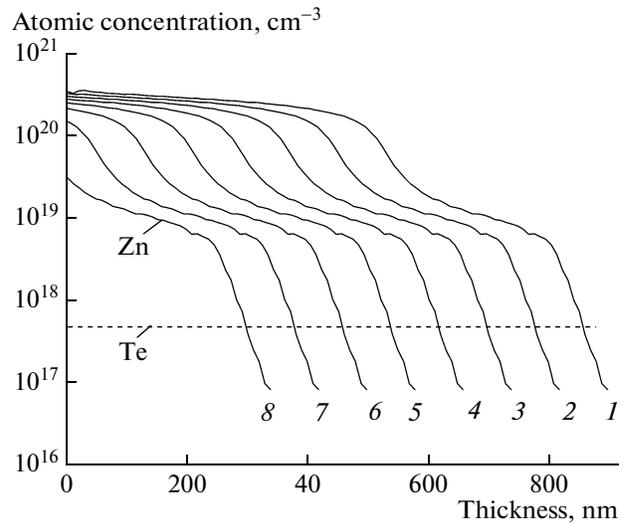
**Fig. 3.** Distribution of zinc atoms in GaSb with an initial thickness of the front  $p$  layer of 850 nm. Thickness of the removed diffusion layer: (1) 0, (2) 80, (3) 160, (4) 240, (5) 320, (6) 400, (7) 480, and (8) 560 nm.
