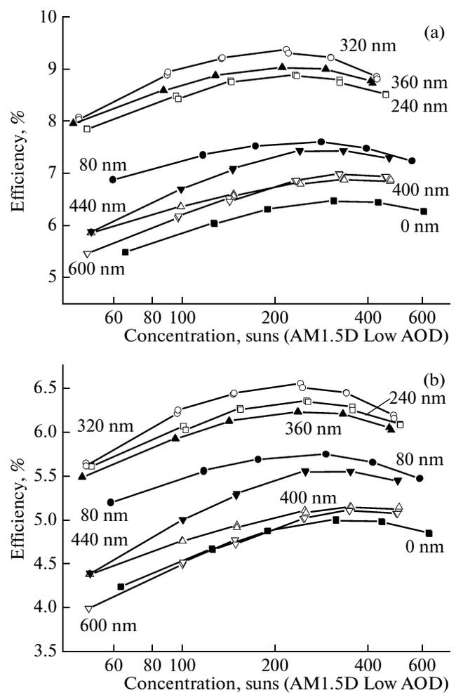
**Fig. 8.** Efficiency vs. the sunlight concentration ratio at various emitter etching depths for GaSb cells exposed to the following sunlight spectrum bands (AM1.5D): (a)  $\Delta\lambda_1 = 500\text{--}1820\text{ nm}$  and (b)  $\Delta\lambda_2 = 900\text{--}1820\text{ nm}$ . “Epi-ready” GaSb substrates from Giredmet.
