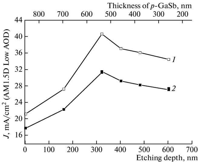
Fig. 5. Photocurrent density vs. the etching depth and emitter thickness: (1) for the internal quantum yield and (2) for the external quantum yield.
