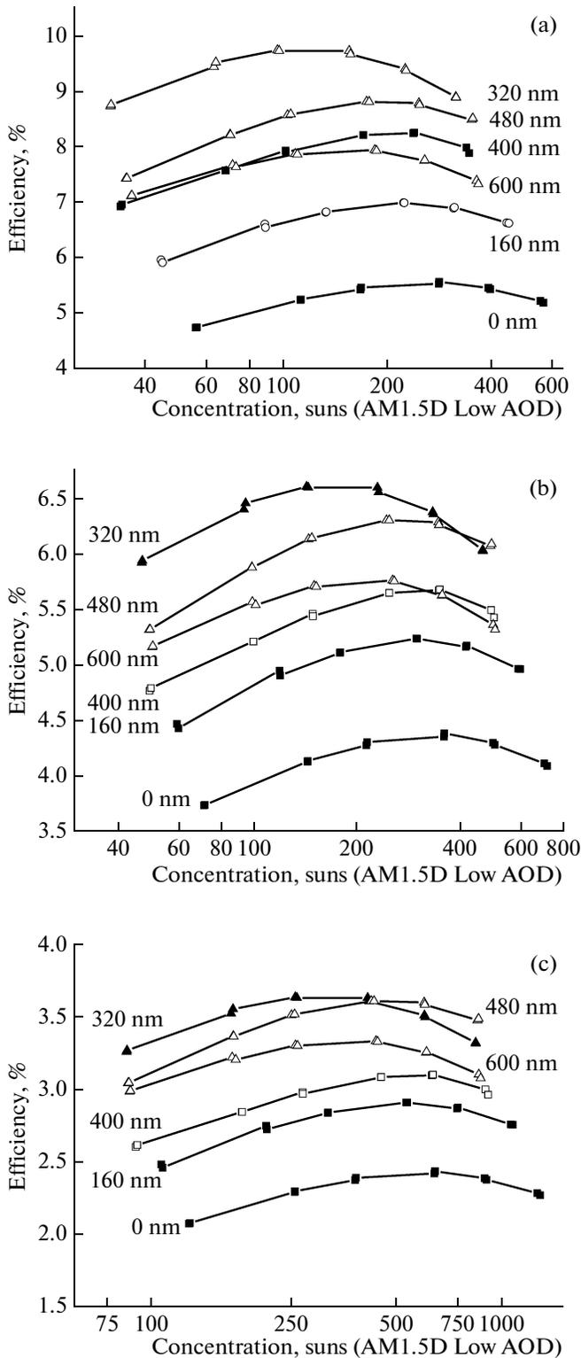
**Fig. 7.** Efficiency vs. the sunlight concentration ratio at various emitter etching depths for GaSb cells exposed to the following sunlight spectrum bands (AM1.5D): (a)  $\Delta\lambda_1 = 500\text{--}1820\text{ nm}$ , (b)  $\Delta\lambda_2 = 900\text{--}1820\text{ nm}$ , and (c)  $\Delta\lambda_3 = 1180\text{--}1820\text{ nm}$ . GaSb ingot from Giredmet, Moscow; wafer cutting and polishing at the Ioffe Physical–Technical Institute.
