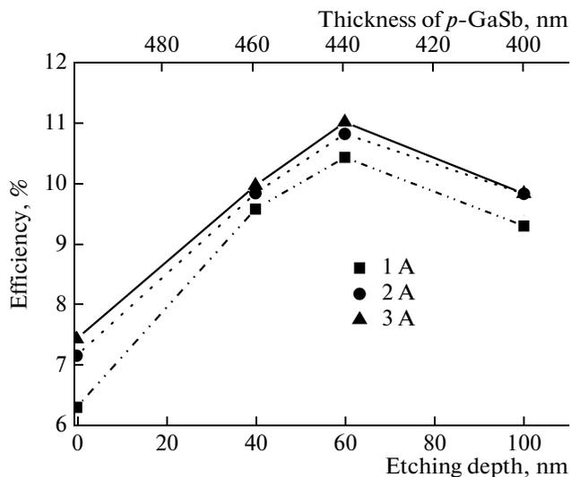
**Fig. 9.** Efficiency vs. the sunlight concentration ratio for GaSb solar cells (AM1.5D,  $1000 \text{ W m}^{-2}$ ) vs. the emitter etching depth at various generated photocurrent densities. GaSb substrates from LETI/DOPT (France) and Ioffe Physical–Technical Institute.
