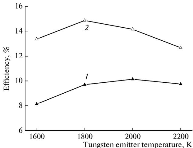
**Fig. 10.** Efficiency of TPV GaSb cells vs. the tungsten-emitter temperature: (1) GaSb structure without thinning of its  $p-n$  junction and (2) structure with a diffusion layer etched to a depth of 320 nm.
