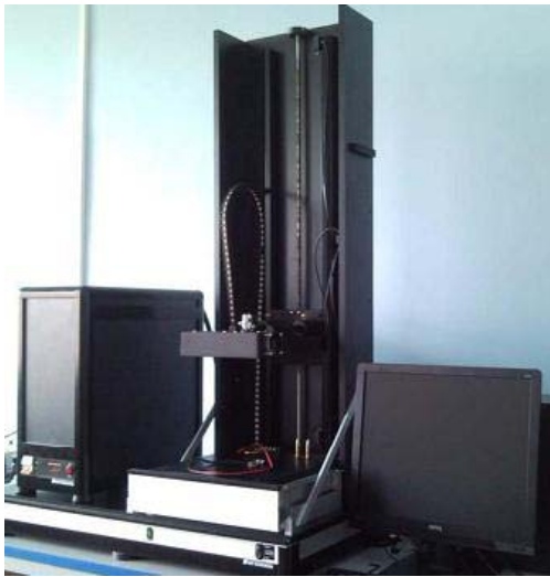
FIGURE 1. Picture of the elaborated solar tester (light protective housing is removed).
