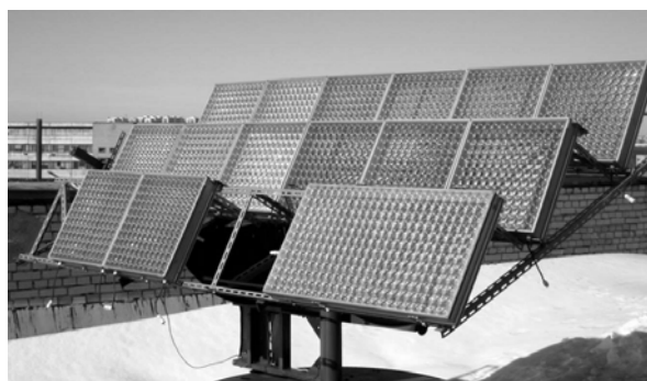
FIGURE 4. HCPV modules 0.5 \times 1.0 \text{ m}^2 and 0.5 \times 0.5 \text{ m}^2 in size on the roof of the Ioffe Institute at outdoor measurements.
