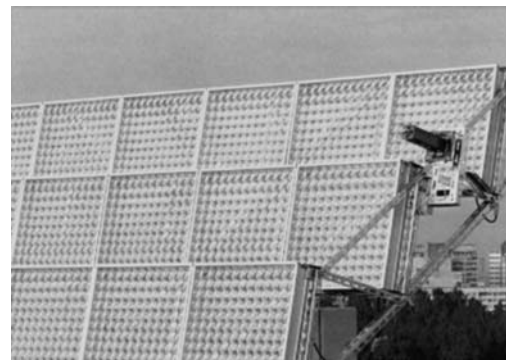
Fig. 8. Modules mounted on the test bench in the Ioffe Physico-Technical Institute.
