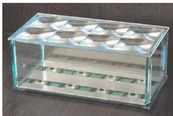
**FIGURE 6.** Picture of one of the 8-lens (60x60 mm<sup>2</sup> lenses) test modules with triple-junction InGaP/GaAs/Ge solar cell (2.3 mm in diameter) and secondary lenses intended for indoor and outdoor tests.
