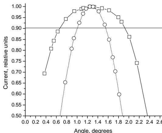
**FIGURE 8.** Widening of the module misorientation curve from  $\pm 0,27$  to  $\pm 0,64$  degree due to introducing the secondary lenses. In both cases, 8-lens concentrator modules with and without secondary lenses were measured (outdoor measurements).
