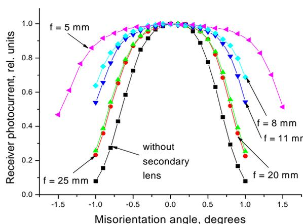
**FIGURE 4.** The results on misorientation angle measurements for a PV sub-module with 40x40 mm<sup>2</sup> primary Fresnel lens, a solar cell 1.7 mm in diameter and secondary lenses of different focal distances  $f$ .
