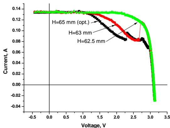
**FIGURE 3.** Illuminated I-V curves of a triple-junction cell with a primary Fresnel lens and a secondary flat-convex lens under illumination from flash solar tester. A distance  $H$  between primary and secondary lenses was varied. The maximum local sun concentration was at the distance of 65 mm (poor I-V curve due to trace of the tunnel junctions), and shortening the distance resulted in defocusing of light (improvement of the fill factors took place).
