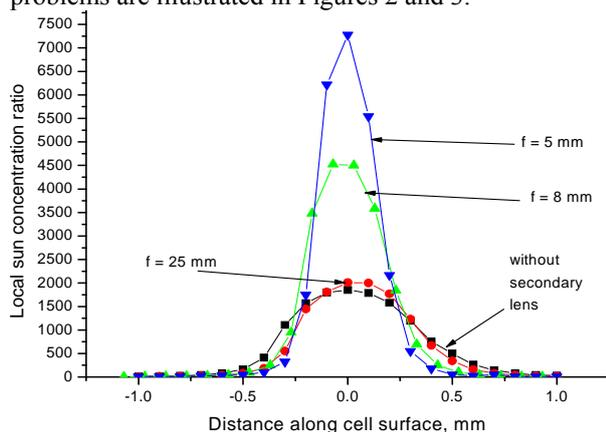
**FIGURE 2.** Local light concentration along the cell surface measured by scanning the focal spot in a PV system with a primary 40x40 mm<sup>2</sup> Fresnel lens and a secondary lens of different focal distances  $f$ .
