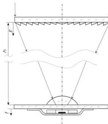
**FIGURE 1.** Optical scheme of an individual solar concentrator submodule. Shown are the planes from which the focal distances  $F$  and  $f$  are measured.
