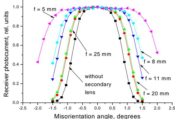
**FIGURE 5.** The results on misorientation angle measurements for a PV sub-module with a 40x40 mm<sup>2</sup> primary Fresnel lens, a solar cell 2.3 mm in diameter and secondary lenses of different focal distances  $f$ .
