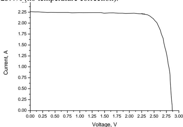
**FIGURE 7.** I-V curve for a 8-lens module with  $60 \times 60 \text{ mm}^2$  Fresnel lenses, cells 2.3 mm in diameter and secondary lenses with  $f = 8 \text{ mm}$ , in illuminating by solar rays incident normal to the module frontal surface. The measured efficiency was 23.4% (no temperature correction).
