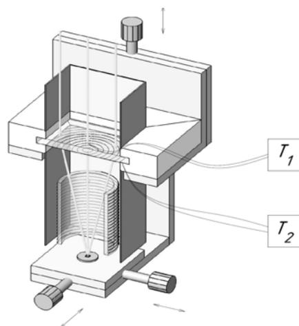
**FIGURE 4.** Lens holder for experiments with variable temperature of the lens.
