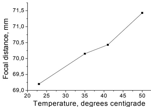
**FIGURE 5.** Dependence of the focal distance on lens temperature. Polymerization temperature at lens profile formation was about 25 C.
