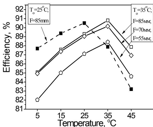
**FIGURE 2.** Calculated dependences of the optical efficiency on operation temperature for lenses with different focal distances  $F$ . Lens area is  $40 \times 40 \text{ mm}^2$ , SC diameter is 1.7 mm.
