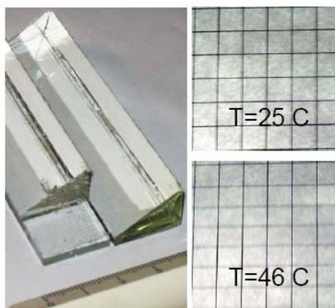
**FIGURE 3.** Macro-model of the silicone prisms on glass base (left) and the pictures of the net with square mesh obtained after reflection from the sloping prism facet at different temperatures of prism material (right).
