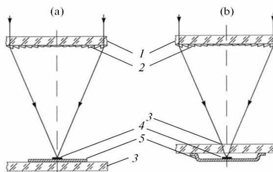
**FIGURE 1.** Optical schemes of the modules: (1) front glass panel, (2) silicone profile of the Fresnel lens, (3) rear glass base, (4) SC, and (5) heat distributing plate.
