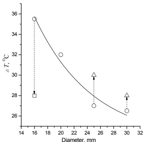
**FIGURE 7.** Overheating  $\Delta T$  of a SC chip compared to the ambient temperature vs. diameter of the heat-distributing copper plate. Circles and triangles refer to the plates 1 and 0.5 mm thick, respectively, which are glued to the glass base 4 mm thick; square refers to the steel plate 1 mm thick. The heat removal area corresponds to the 40 x 40 mm<sup>2</sup> concentrator lens (delivered thermal power is 1 W).
