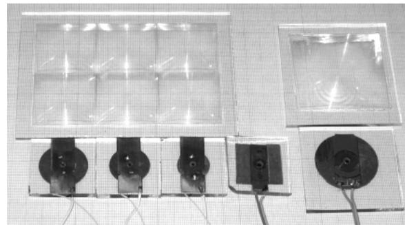
**FIGURE 6.** Pictures of the 40 x 40-mm and 60 x 60-mm Fresnel lenses and physical models of corresponding heat sinks with triple-junction SCs mounted on them.
