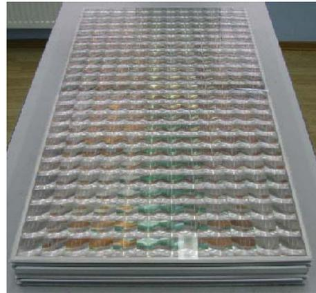
**Figure 12:** CPV module with dimensions of  $0.5 \times 1 \text{ m}^2$  based on 288 submodules of  $4 \times 4 \text{ cm}^2$  each.
