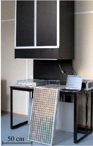
**Figure 13:** Flash solar tester for I-V measurements of the advanced concentrator modules with aperture area up to  $0.5 \times 1 \text{ m}^2$  (shown as well). Collimated light flux with divergence of  $32'$  at 1 sun intensity and spectrum corresponding to AM 1.5d is generated by four flash lamps.
