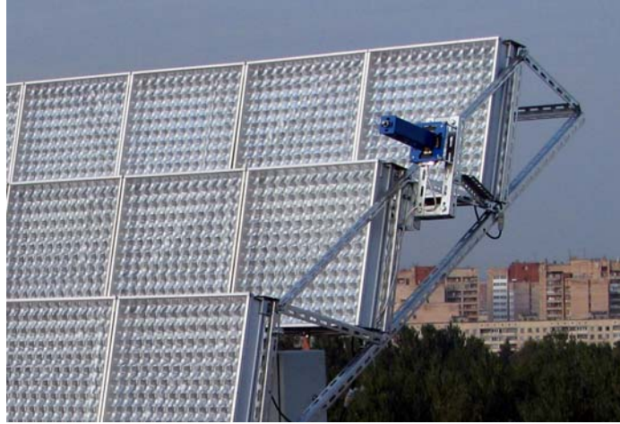
Fig. 2. Photograph of the full-size HCPV modules on a sun tracker (the roof of the Ioffe Institute).
