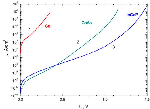
**Figure 4:** Experimental dark current-voltage characteristic of photovoltaic 1-Ge, 2-GaAs and 3-InGaP  $p-n$  junctions laced with corresponding  $V_{OC} - J_{SC}$  characteristics.
