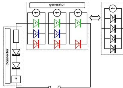
**Figure 1:** Principal electric equivalent circuit of a triple-junction solar cell consisting of generating (photovoltaic) and connecting (connector) parts.
