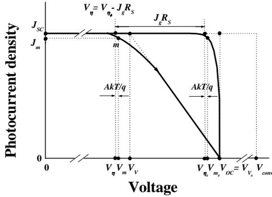
**Figure 3:** Schematic of the light current – voltage (load) characteristic of SCs.
