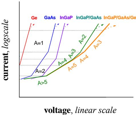
**Figure 2:** Segmental shape of dark current-voltage characteristic of photovoltaic  $p$ - $n$  junctions being a part of a multijunction SC. Segmental shape of dark current-voltage characteristic of dual-junction and triple-junction SCs consisting of the  $p$ - $n$  junctions.
