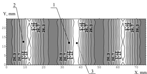
**Figure 6:** Temperature field of the top side of the heat-sink in the maximum power mode: 1, 2, 3 - thermocouples.
