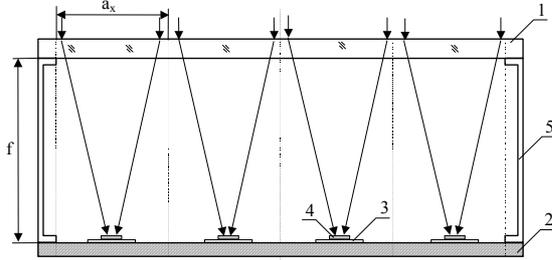
**Figure 1:** Rated module scheme: 1 – linear Fresnel lens panel; 2 – heat-spreading plane; 3 – flexible printed circuit card; 4 – solar cell; 5 – rigid frame.
