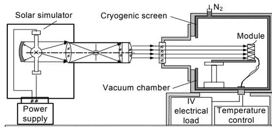
**Figure 3:** Scheme of the experimental bench for the solar module tests.
