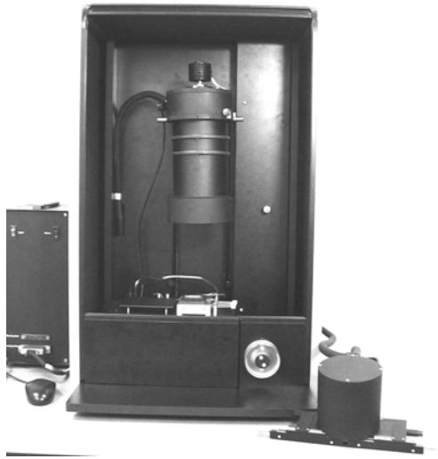
Figure 6: Photograph of the solar simulator reproducing spectrum, intensity, and angle-size of the sun (three-channel illuminating head is shown as well as an optional part of the simulator, see [2]).
