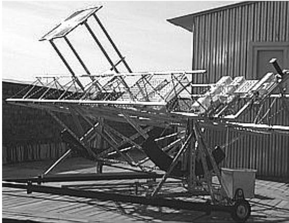
**Figure 5:** Sun tracker with STPV (on the left) and PV concentrator modules (on the right side) based on Fresnel lens concentrators installed at the Ioffe Institute.
